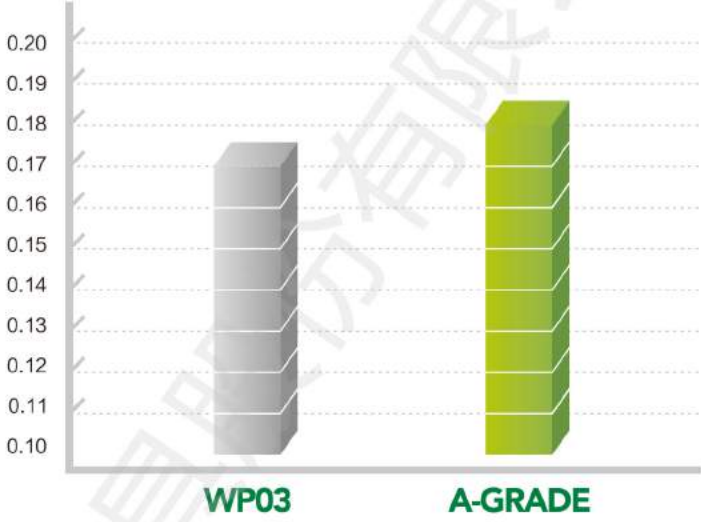
WP03材质和A公司材质磨损值对比 Wear comparison of WP03 and A-GRADE
