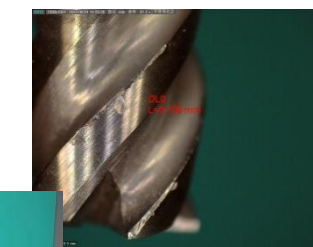
Company A's product is processed for 180min, the flank face is worn after the bottom edge 0.106
