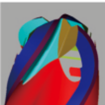
改进前球头容屑槽形状倒 Chip groove before improvement
